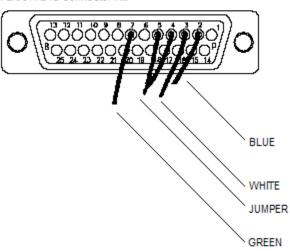
The CHC appears to require wiring as if it were a DTE device. As the FieldServer is A DTE device this implies the cable is NULL Modem like.
